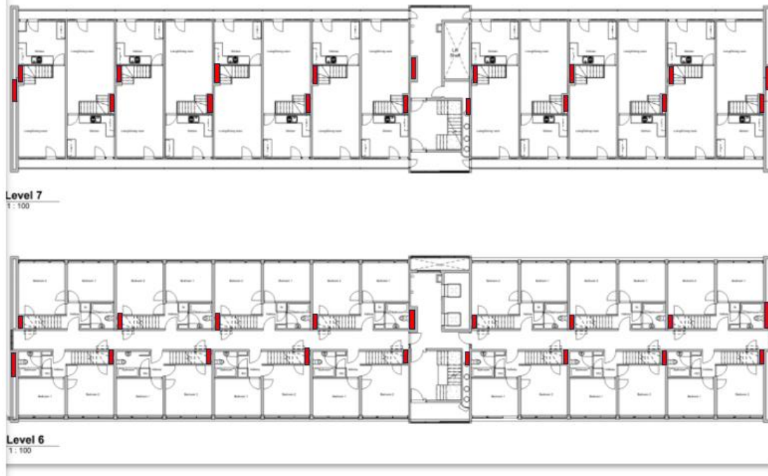
Location of service risers bounded by red boxes (Source: Blakeney Leigh Floor Plan Drawings)
