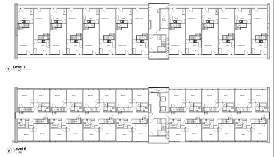
Example floor plans of duplex flats floor levels 6&7 (Source: Blakeney Leigh Floor Plan Drawings)
